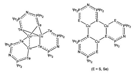
Fig. 9. Structural comparison of: (a)  $[Cu(TeP'Pr_2)_2N]_3$  (23c) and (b)  $[Cu(EP'Pr_2)_2N]_3$  (23a, E = S; 23b, E = Se).
